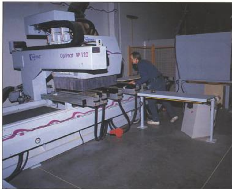
Siewert's Weeke CNC machining center allows an operator to load one part while another is being processed.
