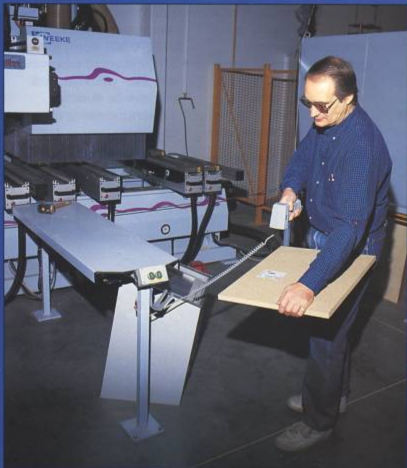
Using a bar coding scanner, an operator quickly sets up the point-to-point portion of a job.
